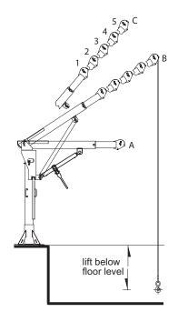
Positions A and C require models equipped with ratchet jack.
