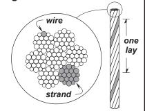
Wire rope assembly must be replaced if more than 6 wires are broken in one lay, or if more than 3 wires are broken in one strand in one lay.
