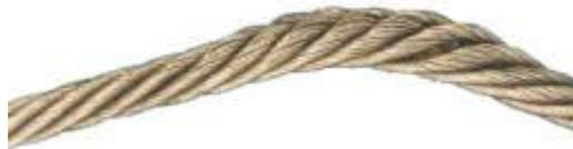
The outer strands of the ropes shall be tight, when the rope is not loaded. In standard and heavy duty ropes the outer strands can have small, visible gap under load. If the gap does not close when the load is released, the rope shall be changed.
