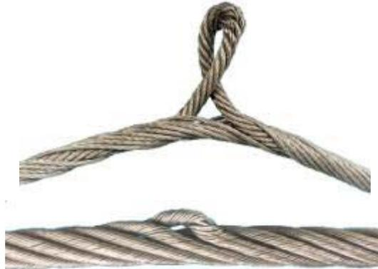
Rope with rise up of core, strand or group of wires shall be changed immediately.
