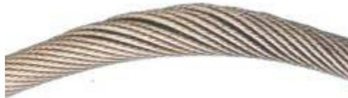
Basket deformation is a result of a difference in length between the rope core and outer strands. Rope with basket deformation shall be changed immediately.
