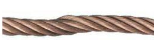
Kink or tightened loop is created by a loop in the rope which has been tightened without allowing for rotation about its axis. Rope with a kink shall be changed immediately.
