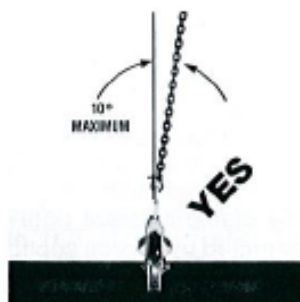
Photograph D Maximum allowable side-loading.
