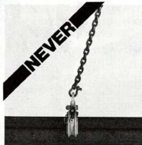
Photograph E Excessive sideloading.
