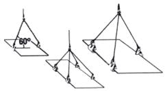
STEEL PLATES: Unless otherwise specified, lifting clamps are manufactured to handle hot-rolled steel plates whose Brinell Hardness does not exceed 300. WARNING: Do not lift plates with coatings or mill scale that prevent the gripping surfaces of the clamp from making positive contact with the base metal.
