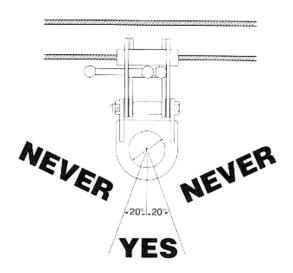
WARNING: When used for lifting, 2 clamps are recommended to insure a balanced lift. When 2 or more are used for lifting, always insure that no single clamps rated capacity is exceeded. Do not exceed maximum angular loading.
