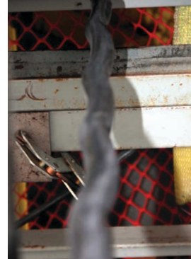
Failing cable due to the “corkscrew” effect
