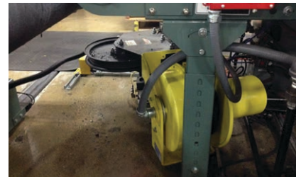
Failing cable due to the “corkscrew” effect
