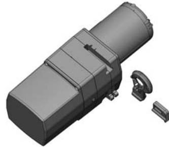
Figure 8B - Single Chain Hook Orientation
