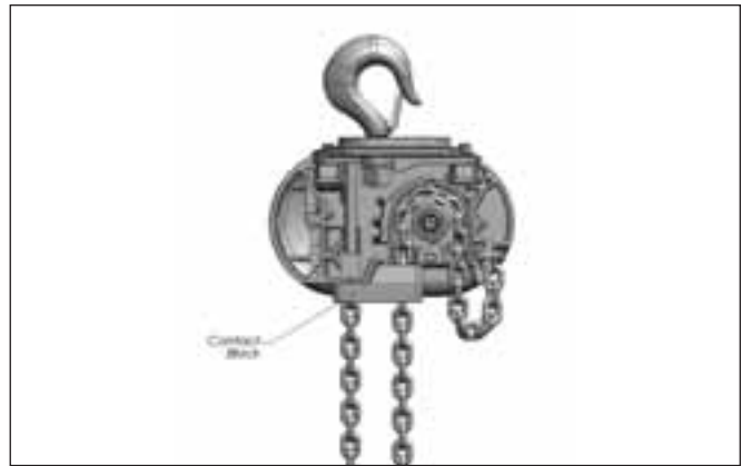
Figure 8. Contact Block Used on Models R, R-2, RR and RR-2
