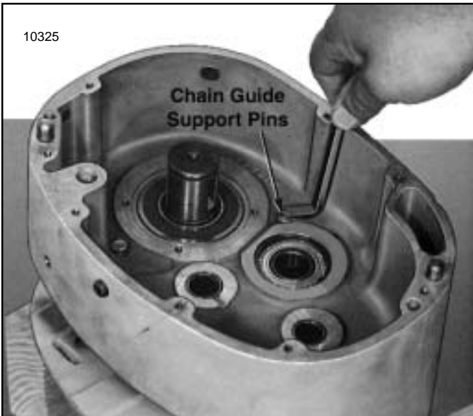
Figure 7-13. Removing Chain Guide Support Pins using Pry Bar
