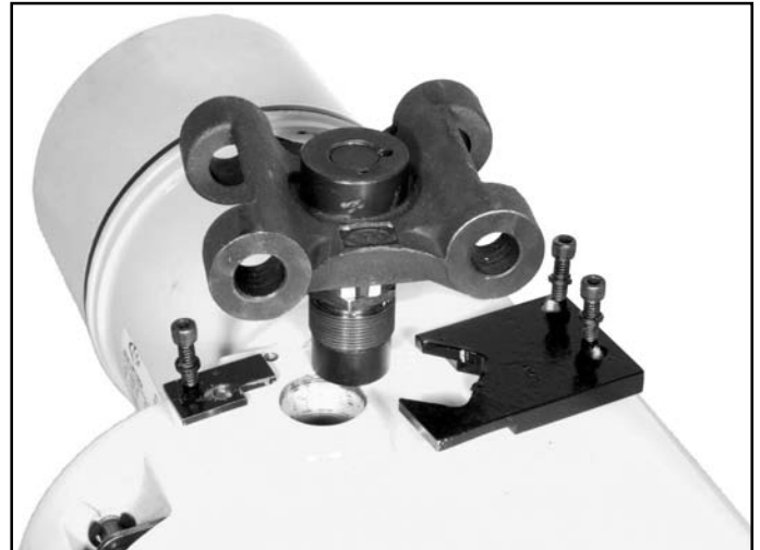
Figure 7-20. Removing Suspension Lug (1/4 through 1 Ton Models)
