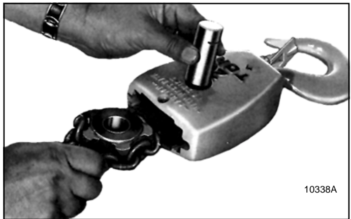
Figure 7-29. Removing Coil Chain and Sprocket on 2 through 5 Ton Lower Block Assembly (Link Chain Model)
