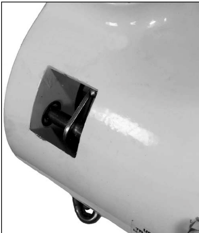
Figure 7-13. Removing Chain Guide Support Pins
