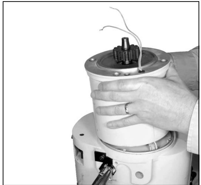
Figure 7-9. Removing Motor Assembly
