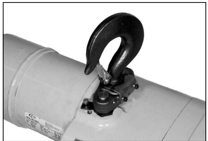
Figure 7-19. View of Upper Hook Assembled to Hoist Frame (2 Ton Models)
