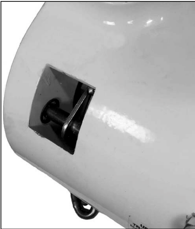
Figure 7-13. Removing Chain Guide Support Pins
