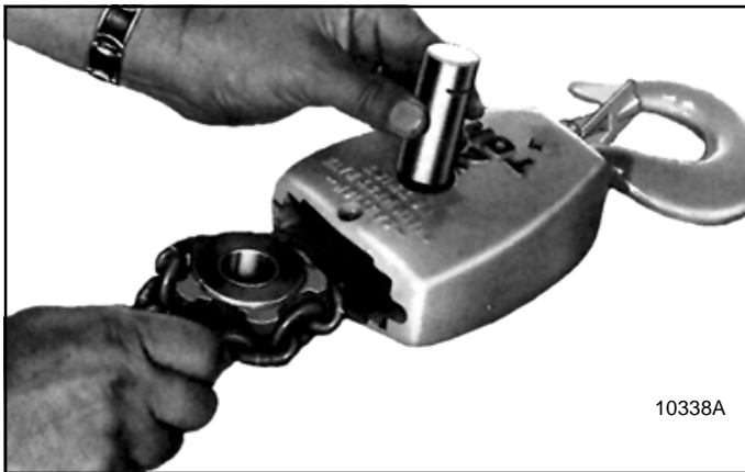
Figure 7-29. Removing Coil Chain and Sprocket on 2 thru 5 Ton Lower Block Assembly (Link Chain Model)
