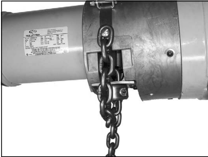
Figure 3-2. Actuator Contacting Stop Tail Chain End of Load Chain
