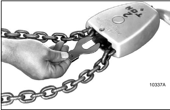
Figure 7-28. Removing Sprocket Pin Lock on 2 thru 5 Ton Lower Block Assembly (Link Chain Model)
