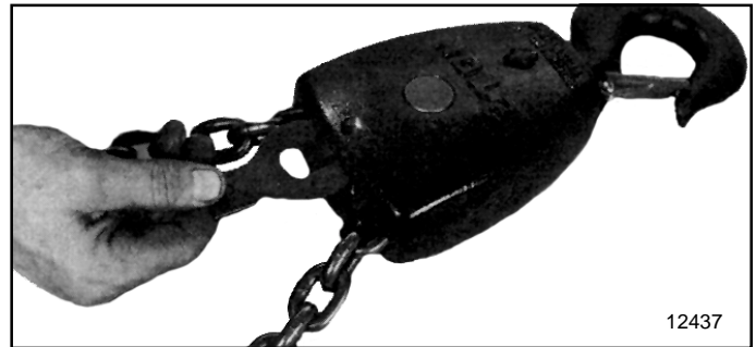
Figure 7-25. Removing Sprocket Pin Lock on Double and Triple Reeved Lower Block Assembly.
