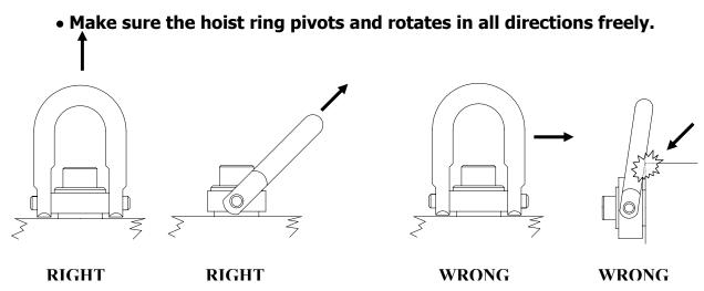
**Important**: The load on each hoist ring is not simply total weight divided by the number of hoist rings. The resultant force can be significantly greater at shallow lift angles and with unevenly distributed loads. See the example below.
