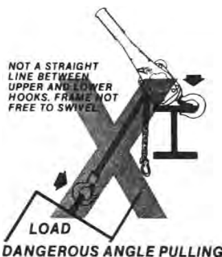
Figure 4 - Pulling at an Angle
